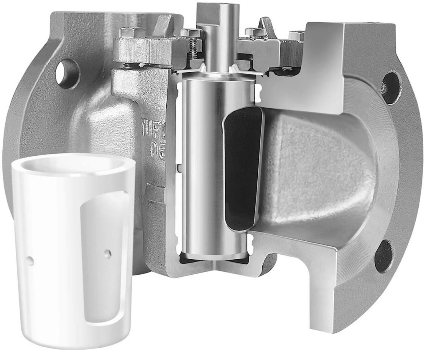
Trouble-free sealing is provided by the large, full-circumferential PTFE sleeve. No ball or gate valve can match this sealing capacity.
